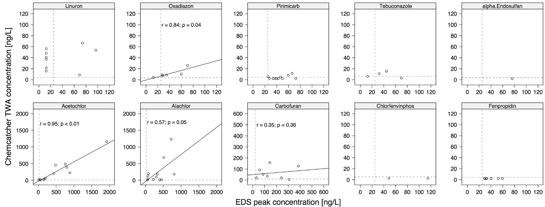
Figure 4: Relationship between the Chemcatcher<sup>®</sup> TWA concentrations and the EDS peak concentrations in 16 agricultural streams, for single compounds. Observations that were below LOQ for both sampling methods were excluded from analysis. Dashed lines indicate LOQ.  $r$  = Pearson's correlation coefficient. Regression lines are shown for > 3 observations above LOQ for both methods.
